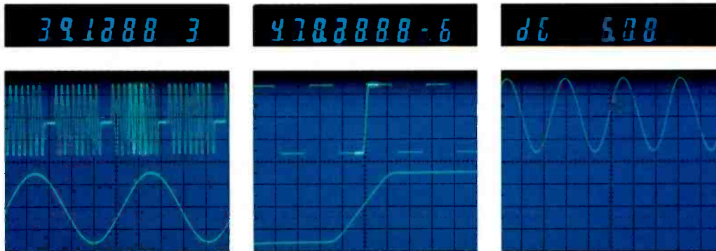
Gated frequency measurement. B sweep triggering during the intensified portion of the A sweep. Intensified portion frequency is measured with the counter/timer/DMM.
